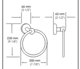
Maximum dimensions - 220 x 200 x 53 mm Distance from the wall - 62 mm Snap flange cover - Ø 53 mm Ring - Ø 200 mm
